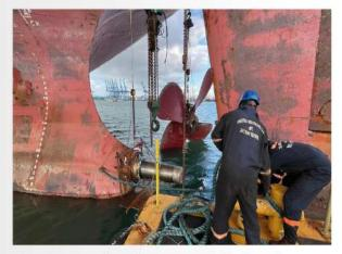
The client ordered a new tail shaft and a new set of connecting bolts 12 pieces and 4 spares for the flywheel connection.
