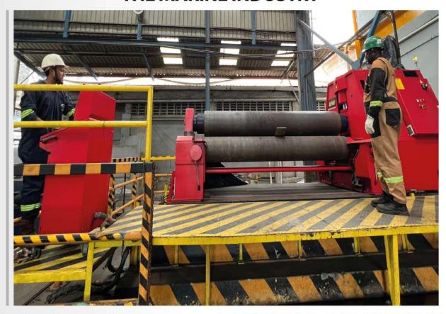
Talleres has invested in a new Davi 3-roll variable-axis plate rolling machine, an accurate tool for plate bending. It features motorized rolls, precise positioning, and a sturdy frame for enhanced performance.
