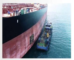
Last month, a Panamax oil chemical tanker suffered a collision during her northbound transit at the Panama Canal. Due to the heavy contact on her port side shell plate, the plate and internal structural members were ruptured and buckled.
