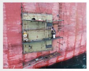
Also, web frames 81 and 82, which were heavily damaged, had to be renewed along with affected longitudinal, steel brackets, and stiffeners.
