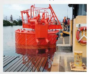
SBM was towed to Colon and at the Panama Canal facilities, Talleres performed deep dry-docking jobs including welding jobs, blasting, painting.
