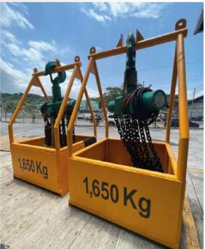
Talleres has invested in heavy lifting pneumatic chain falls to perform major repairs and service outside and inside the vessels at the Panama Canal Area. From Propeller to Rudder removal for repairs to rigging and lifting of vessel engines and machinery from engine rooms. Talleres is equipped to deal with exponential tasks and challenges, 24/7!
