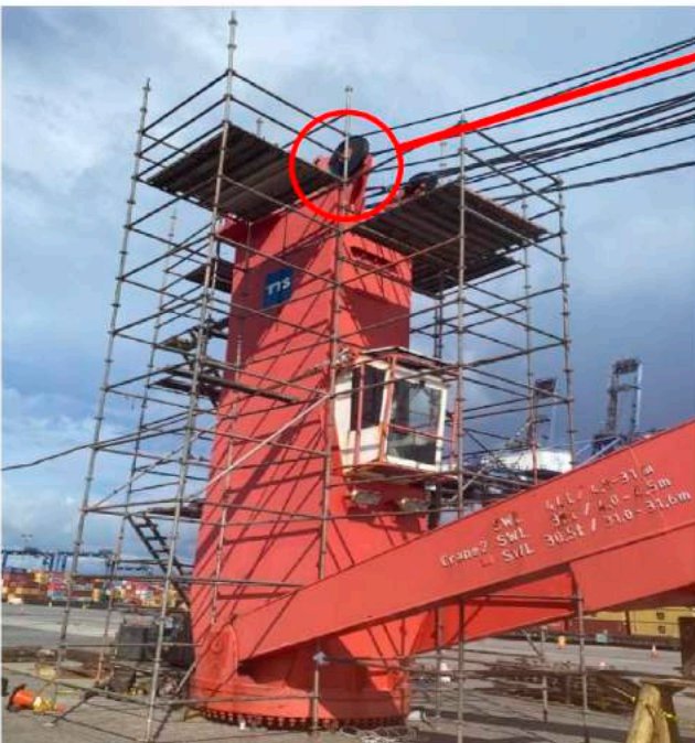
Damages on top tower sheaves, sheaves support
