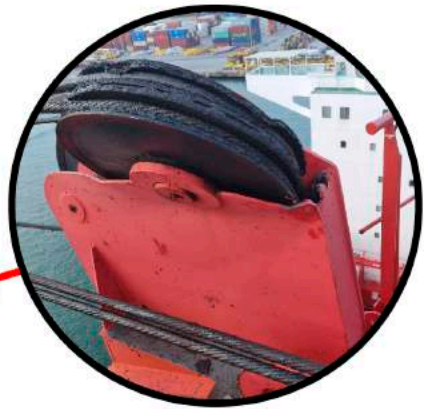
Damages on top tower sheaves, sheaves support
