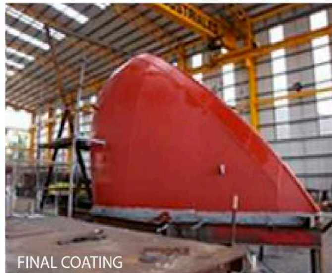
FABRICATION OF THE BULBOUS BOW IN OUR WORKSHOP
